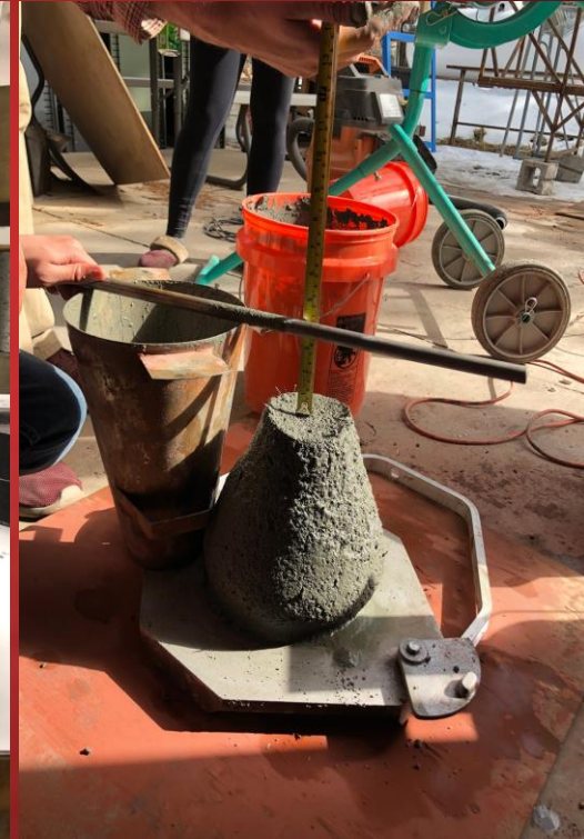
Figure 8: Slump test on practice pour day.
