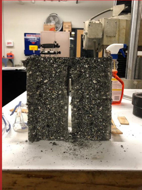
Figure 7: Tensile break showing clear failure of aggregates.
