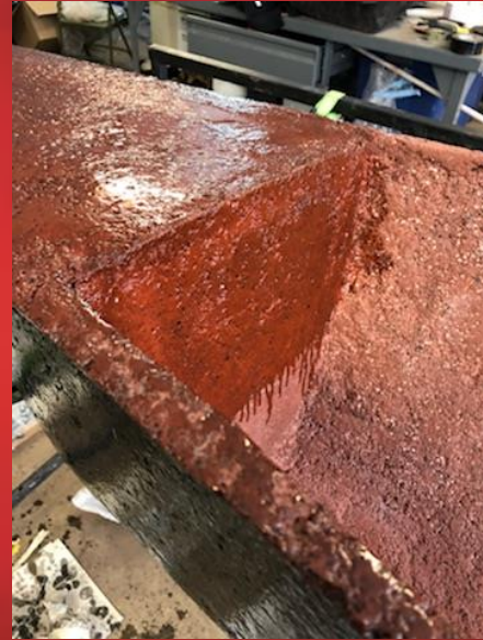
Figure 47: Applying 1 st layer of sealant to VolCanoe.
